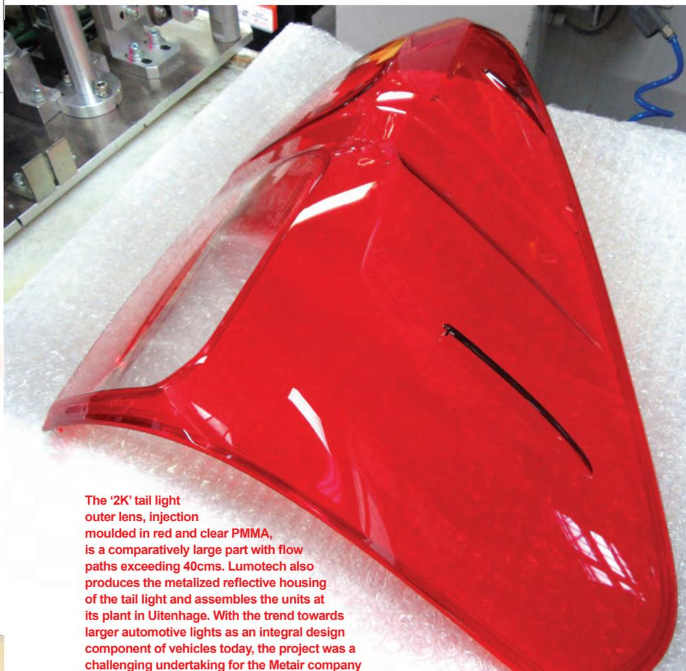
The '2K' tail light outer lens, injection moulded in red and clear PMMA, is a comparatively large part with flow paths exceeding 40cms. Lumotech also produces the metalized reflective housing of the tail light and assembles the units at its plant in Uitenhage. With the trend towards larger automotive lights as an integral design component of vehicles today, the project was a challenging undertaking for the Metair company
